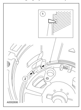
59. Install the center shaft thrust bearing (No. 3).
